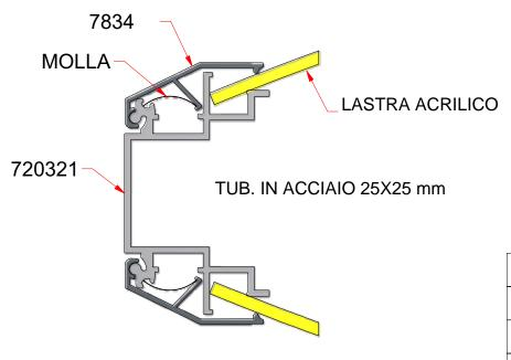
CALOTTA 50 cm - SVILUPPO LASTRA = 50.1 cm - LUCE = 47.5 cm CALOTTA 60 cm - SVILUPPO LASTRA = 59.6 cm - LUCE = 57.0 cm CALOTTA 70 cm - SVILUPPO LASTRA = 70.0 cm - LUCE = 67.4 cm
